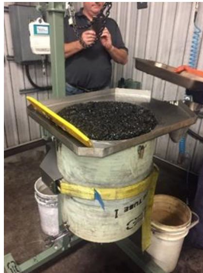
The first slice of coal is ready to be removed from the cylinder. It has been pushed up from the bottom and will be scraped off into a weighing container for Apparent Relative Density test.
