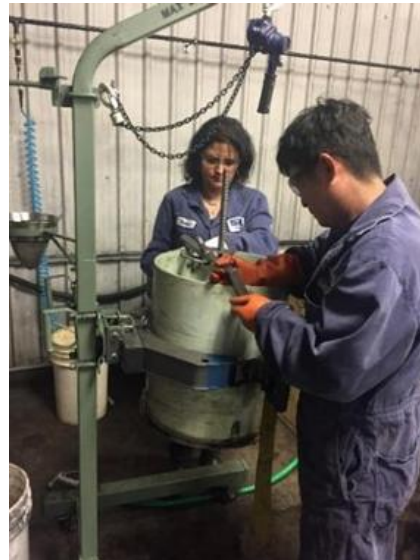
Technicians getting ready to invert the jig tube holding jiggled coal.
