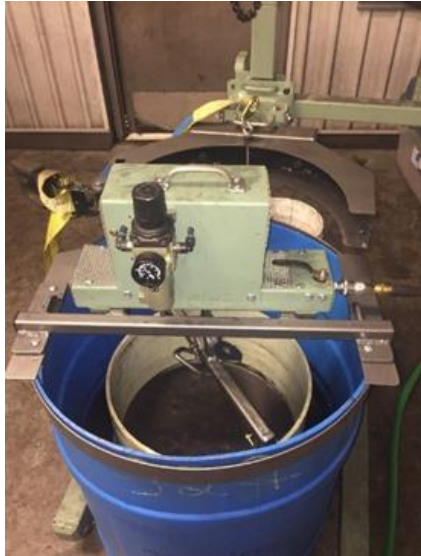
Roben Jig tube filled with coal and water and ready to be jiggled.
